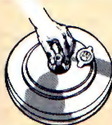
3 Inserting Fuze In Mine.
