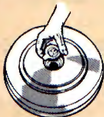
1 Removing Arming Plug From Mine.
